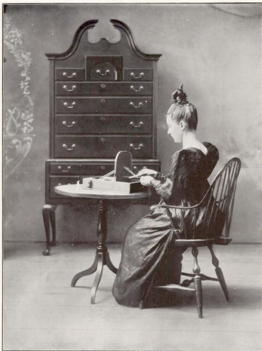
LOOM WITH HEDDLE FRAME FOR WEAVING SILK BRAID.
